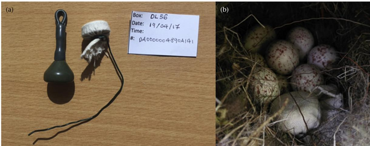
**Figure A1.** iButton set-up for incubation data collection. (a) Preprogrammed iButton wrapped in fabric and attached to wire (weight 28.35 g) and iButton field label. (b) Detail of a nest cup with the iButton device positioned among great tit eggs.
